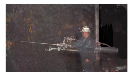
PHQ provides a complete column bar set-up for the Bazooka drill. The heavy wall tube column bar is held in place by the powerful MineJack Ratchet Jack providing a very solid and rigid base for the Bazooka drill cylinder to push against when drilling or retracting drill rods from the hole.
