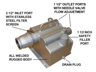
SAFETY TIP: Always shut the air off and bleed the pressure out of the compressed air system containing the F61 Lubricator before attempting to adjust the needle valve flow settings in the F61. The needle valve can unscrew far enough to blow out of the thread holding it in and become a projectile under pressure.
