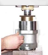
81. When a Chuck Gear (49) is returned to the drill shop with a worn Chuck Bushing (50) the chuck bushing should be removed using the fifty ton hydraulic press in the shop. Examine the Chuck Gear for wear and if it is still in satisfactory condition press in a new Chuck Bushing (50) using the fifty ton shop press. The repaired assembly can be used to replace a worn or damage assembly at the underground drill site.
