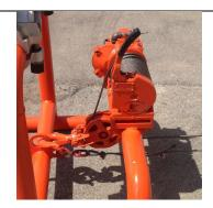
The AW80 Hoist is controlled by a four way valve assembly. The valve assembly is mounted to bracket fabricated from channel steel with a handle. The channel steel fits snugly over the arm where the Remote Control Panel is mounted. The bracket and valve can easily be removed from the arm by lifting upwards, and is fully portable to allow the driller to move around the drill sled setup to a safe location to operate the AW80 hoist to move the sled.
