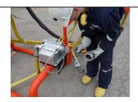
After examining the lubricator filter and checking the oil is sure that the filler cap is securely tightened with a mine wrench.
