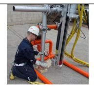
Once the wooden blocks are in place the miner loosens the nuts on the universal clamp holding the upright column bars elevated from the ground. One must take care to loosen only the nuts that will allow the column bar to drop down onto the wooden block. The other two nuts on the same universal clamp are holding the column bar upright and if loosened would allow the whole setup to rotate on the horizontal arm and fall out of place.
