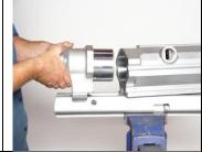
78. To install the Front Cylinder Washer (31) into the Cylinder (43) the two parts should be slid into a short length of guide shell (from the Feed Assembly) and tapped with the rubber hammer to set the two parts together with correct alignment of the ways of the two parts before the Front Cylinder Washer is press fitted into the Cylinder (43) using the fifty ton hydraulic press in the shop
