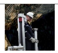
Pull up on the inner tube until the top of each of the column bars is just below the back of the tunnel or stope and inert the bolt through the hole in the outer bar and the corresponding hole in the inner bar. Thread on the nut to be sure the setup is safe.
