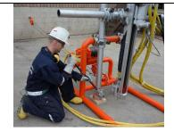
There is no need to tighten the nuts that were loosened to drop the column bars as the drill set-up is not resting securely on the two column bars. All other nuts on the drill set-up should now be tightened to be sure that the entire setup is very rigid.
